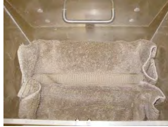
Figure 2: Bag wrapped in towel, leaving half the towel with no heat source
