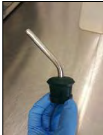
Figure 2: Bung and sipper assembled.
