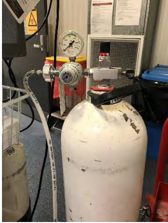
Fig 2. Medical Oxygen Gas Cylinder with Regulator on Trolley
